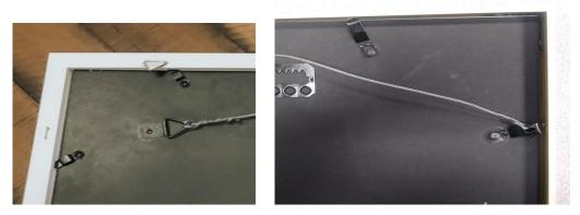
For store bought wood frames, eye hooks or d-hooks need to be screwed into frame and wired.
